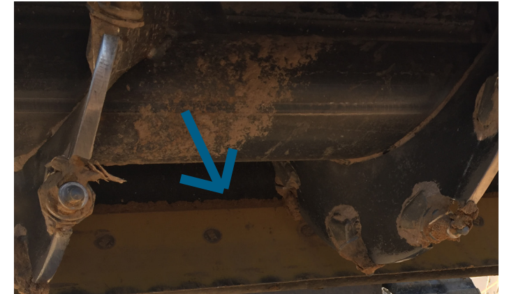
Mid mounted grader blade that rides between the trimmer and the rolling drum
